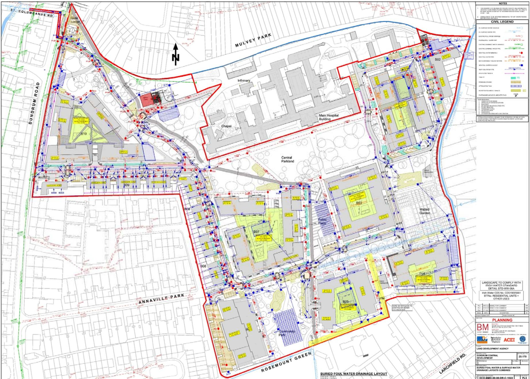
Figure 8. Buried foul and surface water drainage network
