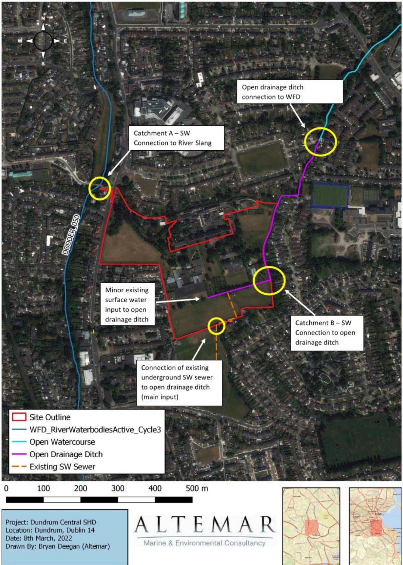
Figure 16. Outline of hydrological connections between waterbodies
